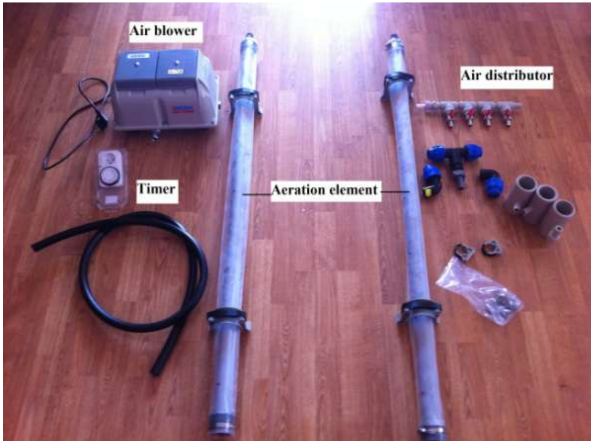
Picture 1, Biological waste water treatment system components
