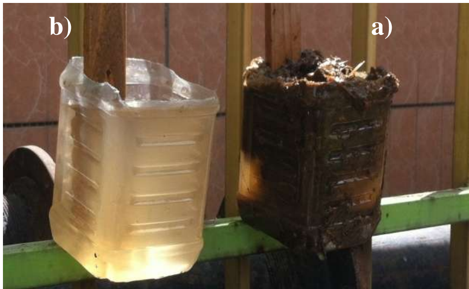
Picture 16, The Biological sewage treatment system in the are of Kabul Municipality headquarters (for 20 -25 people), Samples of taken water from different stages of filtration and purification, a) The input sewage, b) water after purification and filtration
